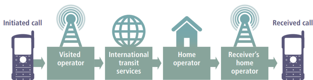
Figure 1: Visualization of the connection of a roaming call to a domestic number
